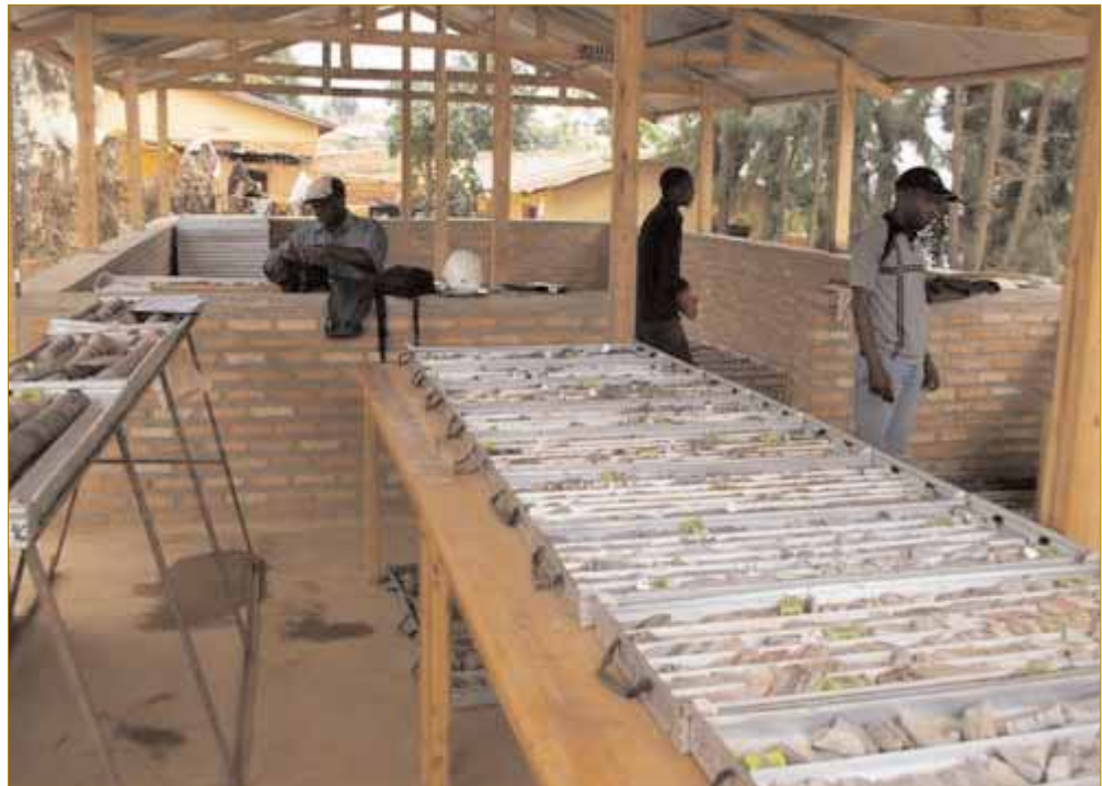
Borehole core being logged
